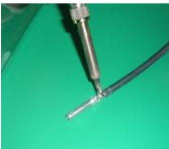
For ensure the conductor and cable is sufficiently strong after crimped, we recommend to use tin solder to prevent connection break off.
